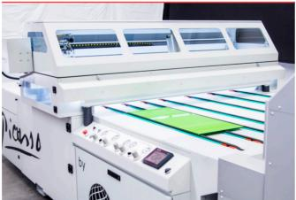
Glass is detected by sensors to measure both length and width automatically.
