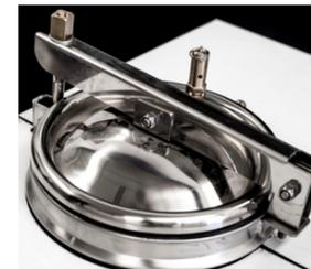
Perfect for recycling your dirty solvents, reclaiming up to 80% reusable material. Dirty solvents are poured into the container. Machine is set to the required temperature and the recycled solvent is fed into a clean container leaving the inert waste in a disposable bag.
