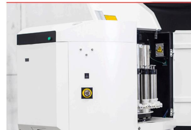
Easy access to canisters for refill of pigments. Suitable for CR water based and solvent based systems.
