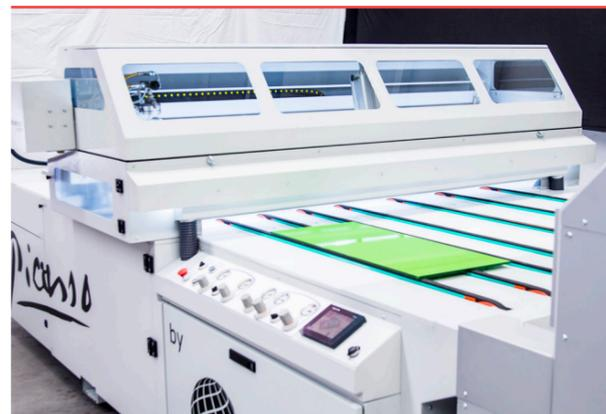
Glass is detected by sensors to measure both length and width automatically. The Ultrasonic sensors are protected by anti-dust air chamber to keep them clean. Suitable for rectangles, circles and irregular shaped glass
