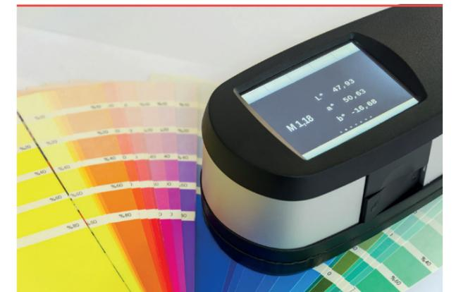
System uses Creative Resins Colour Match software with over 15,000 colours. Connect our spectrometer to scan a sample and dispense the closest matching colour from the extensive colour library.
