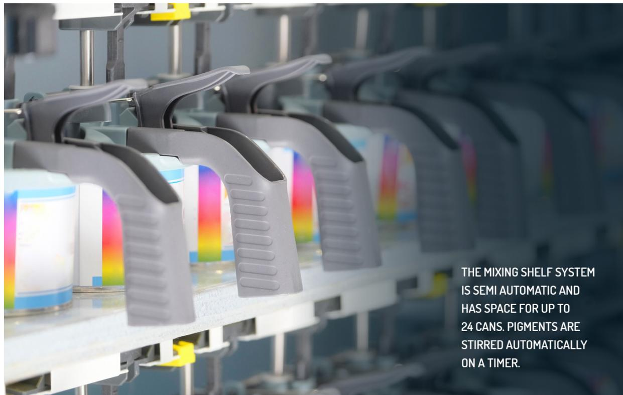
THE MIXING SHELF SYSTEM IS SEMI AUTOMATIC AND HAS SPACE FOR UP TO 24 CANS. PIGMENTS ARE STIRRED AUTOMATICALLY ON A TIMER.
